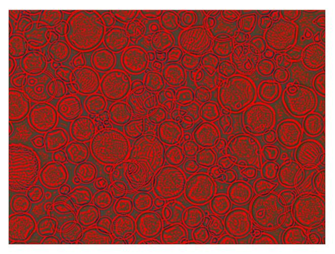
An ImageJ software gure of Alginate microgels generated using a newly developed air-assisted co-axial device (ACAD). These microgels have various potential applications such as encapsulation and delivery of cells and fabricating cell-laden structures via 3D bioprinting.
