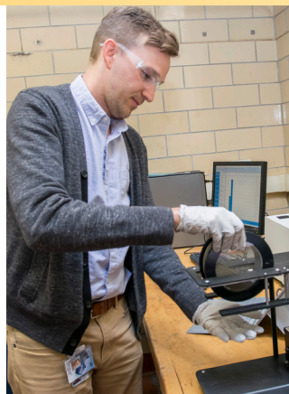
Left: Ph.D. candidate Andrew Iams demagnetizes an additive manufacturing powder feedstock sample prior to performing rheological and charge measurements on a powder rheology system.
